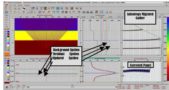
Figure 3. Epsilon correction at the third layer: true 0.2, background 0.125, residual 0.06
