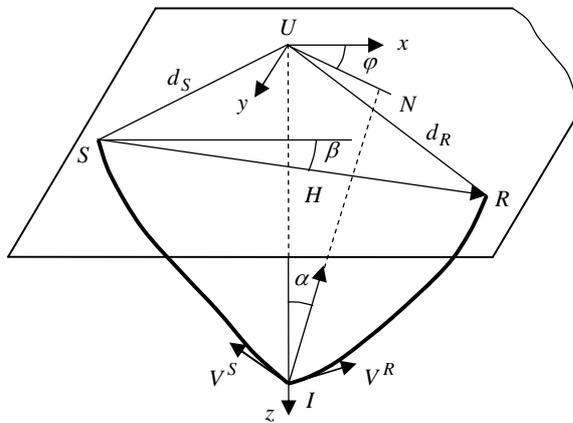
Figure 1. Boundary value ray tracing
