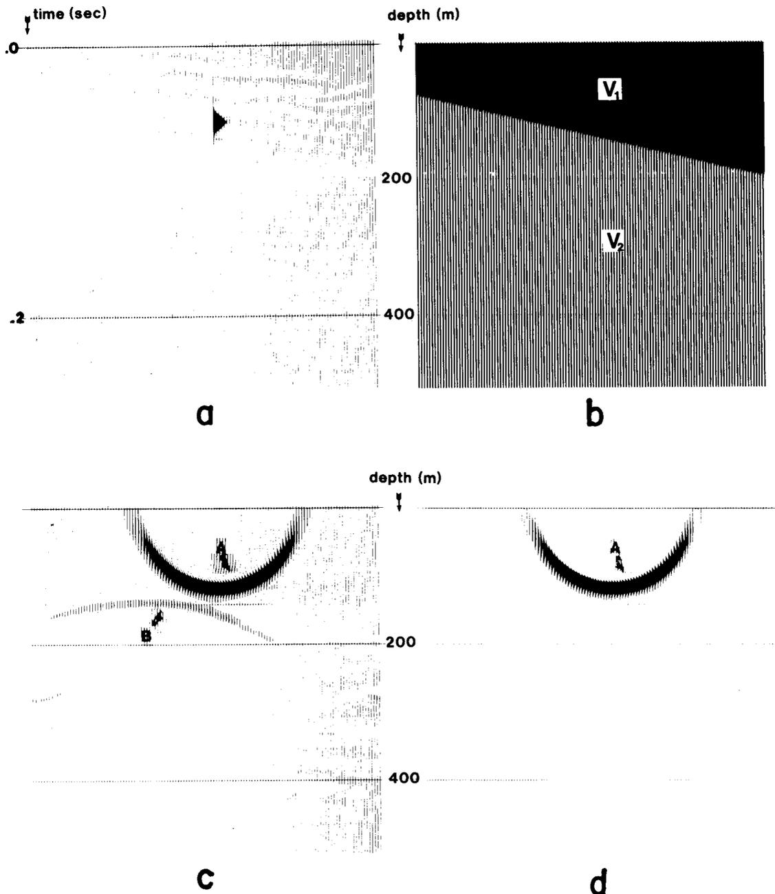
FIG. 2. (a) A time section containing a single spike. (b) Velocity model  $V_1 = 2000$  m/sec.  $V_2 = 1000$  m/sec. (c) Migrated section based on equation (3). (d) Migrated section after the elimination of downgoing energy at time  $t = 0$ .
