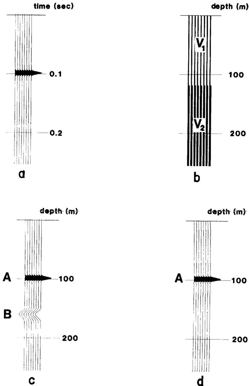
FIG. 1. (a) A one-dimensional time section containing a single event. (b) Velocity model  $V_1 = 2000$  m/sec,  $V_2 = 1000$  m/sec. (c) Migrated depth section based on equation (3). (d) Migrated section after the elimination of downgoing energy at time  $t = 0$ .
