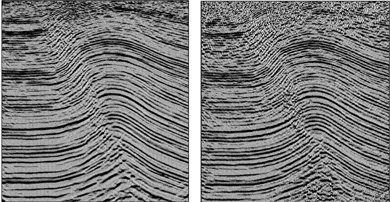
*Figure 3: PSDM of the Beaver Creek field. Left: Kirchhoff summation PSDM. Right: High frequency (60 Hz) Reverse Time Migration (RTM) PSDM.*
