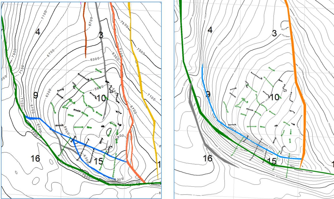
Figure 1. Beaver Creek Field structure based on PSTM data (Left) and PSDM data (Right). Only wells utilized in the CO<sub>2</sub> flood are posted.
