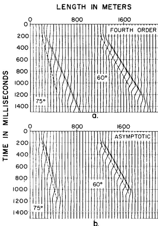
FIG. 5. Magnified views of the migrated sections shown in Figure 4.
